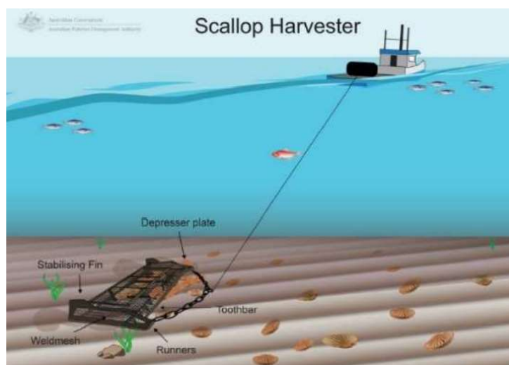
Figure 14. Scallop dredge method diagram (image source: afma.gov.au ).
