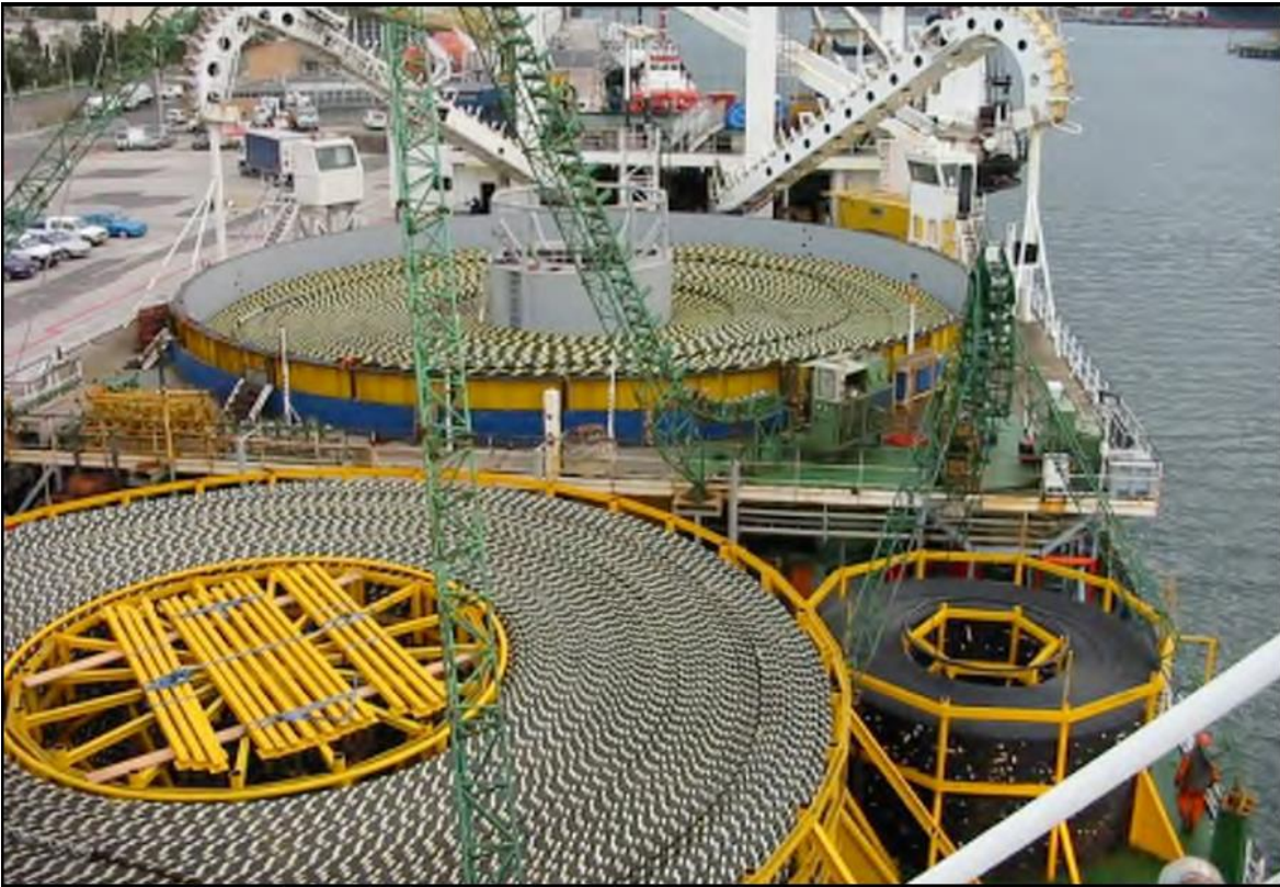
Plate 4.2: CIS Giulio Verne with HVDC cable turntables and an optical fibre cable tank
