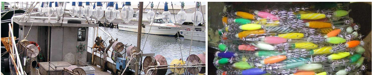
Figure 12. Left; Deck of an Australian squid jigging machine showing arrangement of jigging machines. Right; Commercial squid jigs wound around a jigging machine drum.
