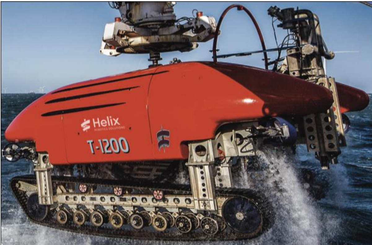
Plate 4.6: Example of a cable trencher – the Helix T-1200 Trencher™
