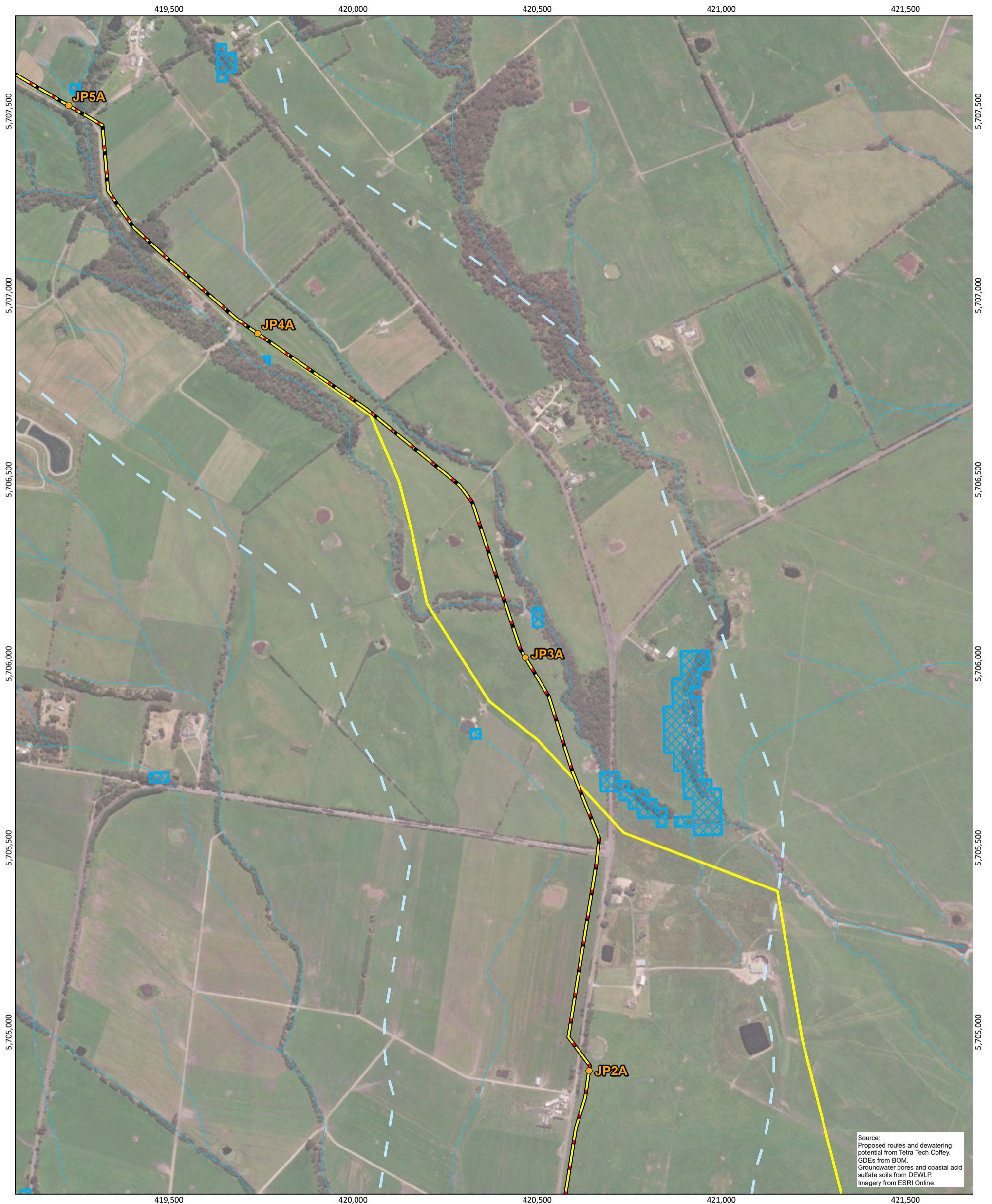
Figure 7.1 - Onshore area likely requiring dewatering (map 2 of 29)
