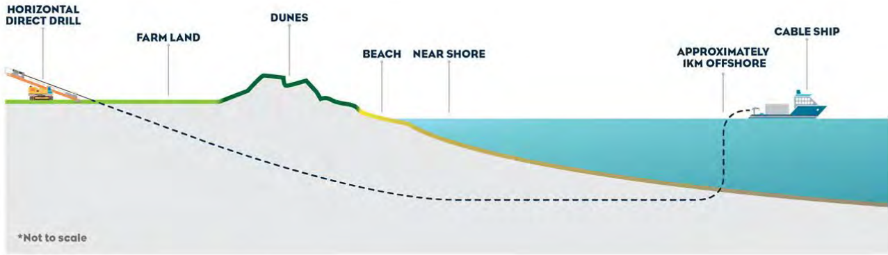
Figure 4-1 Indicative shore crossing construction
