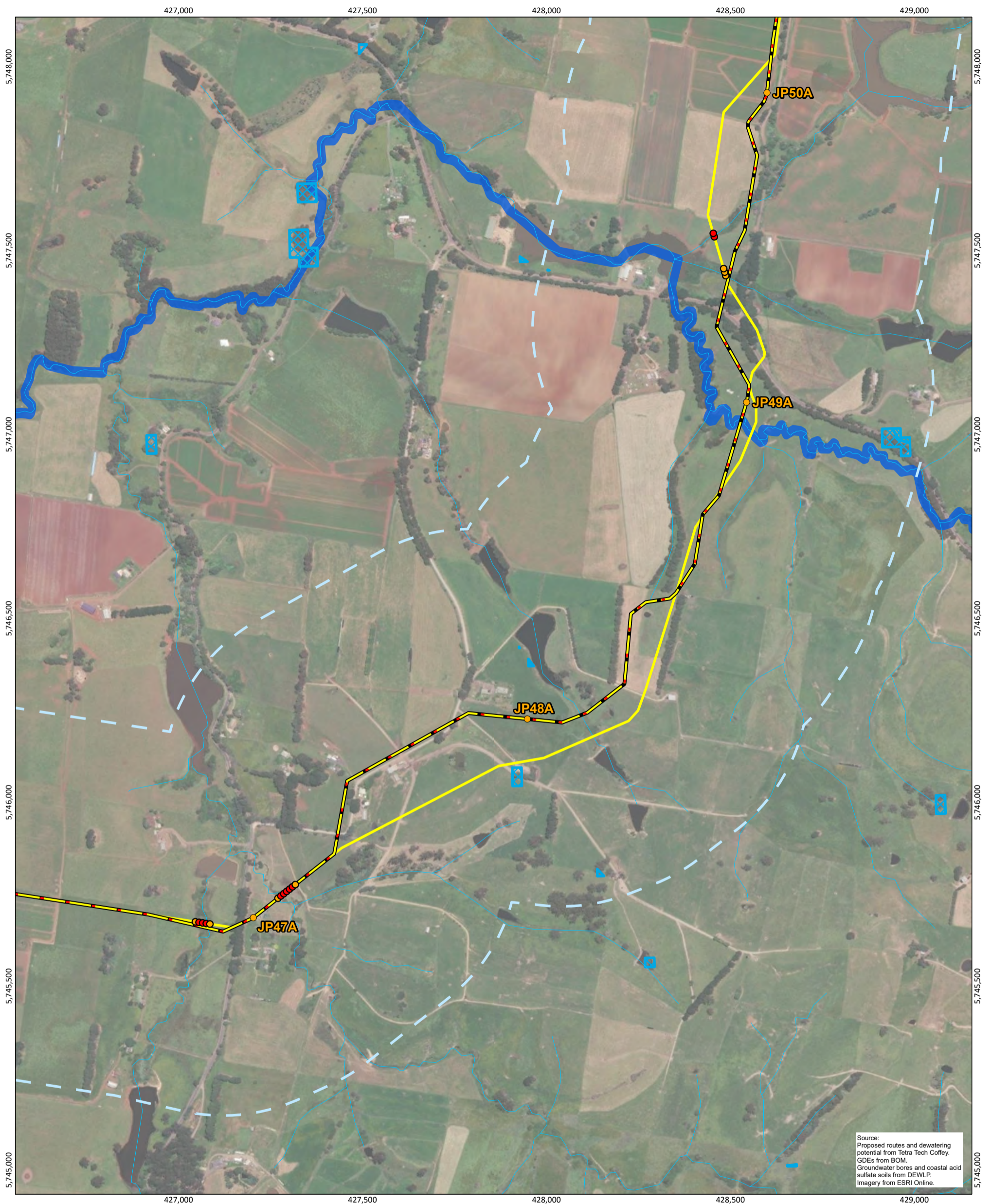
Figure 7.1 - Onshore area likely requiring dewatering (map 18 of 29)
