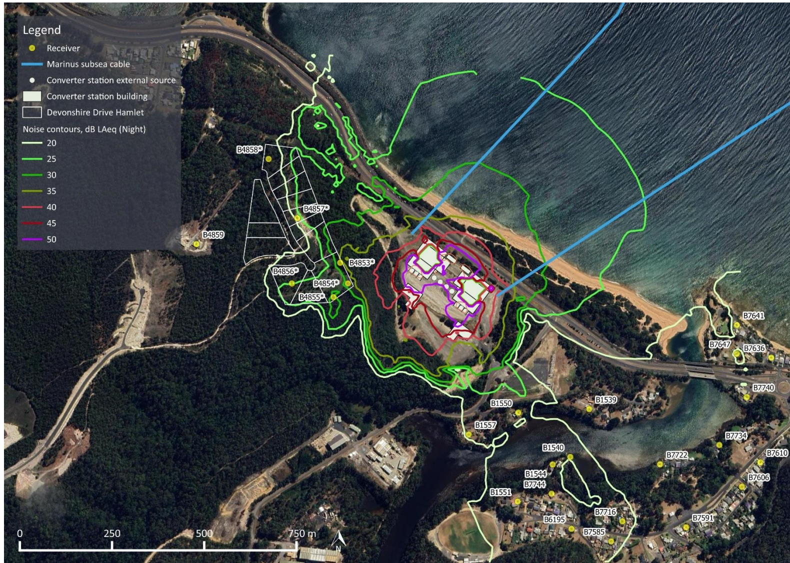
Figure 16: Heybridge converter station site – predicted noise contours for typical night operation, dB LAeq
