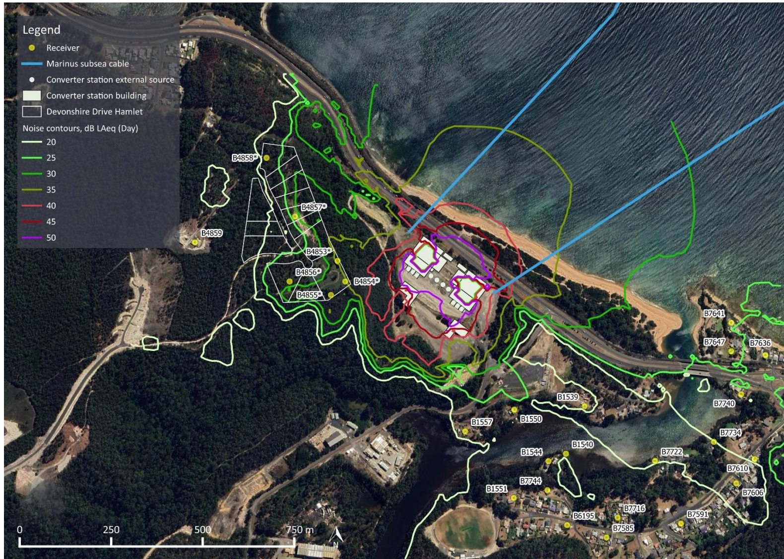
Figure 15: Heybridge converter station site – predicted noise contours for typical day operation, dB LAeq
