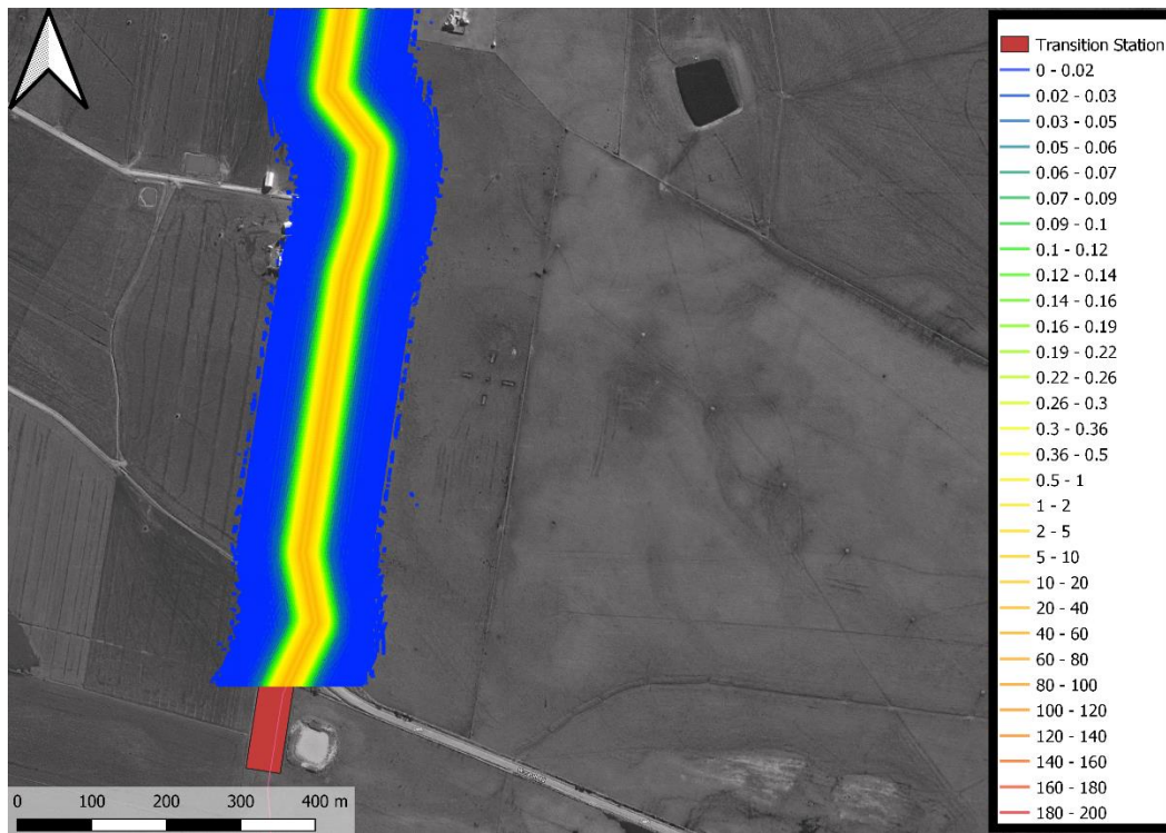
Figure 7-28: Calculated magnetic field distribution in the vicinity of the HVDC land cable – 0.5 m inter-cable spacing
