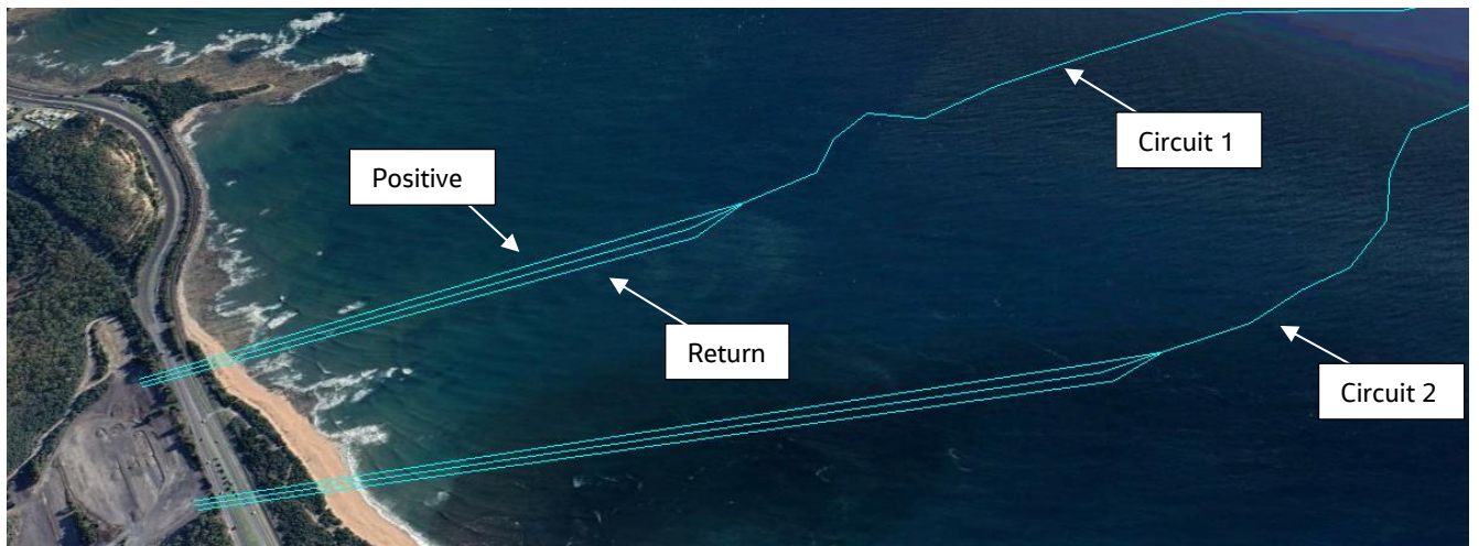
Figure 5-2: Non-uniformity of cables at the Tasmanian shoreline
