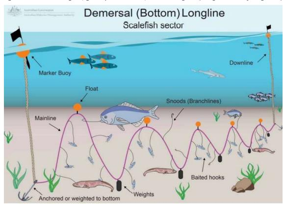
Figure 9. Demersal longline, scalefish sector, method diagram (image source: afma.gov.au).
