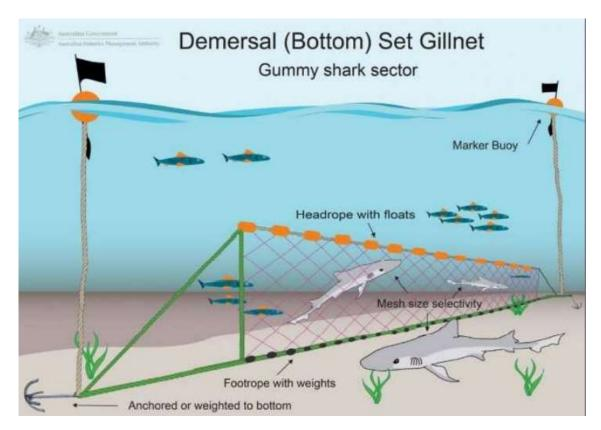
Figure 7. Demersal gillnet method diagram (image source: afma.gov.au)
