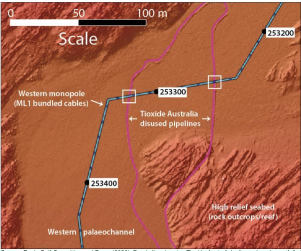
Source: EnviroGulf Consulting and Fugro (2020). Purple line denotes Tioxide Australia's disused marine outfall pipelines. Blue line denotes the ML1 bundled cable within the western palaeochannel. White boxes indicate the crossing locations but not the area of rock fill or concrete mattress cover.
