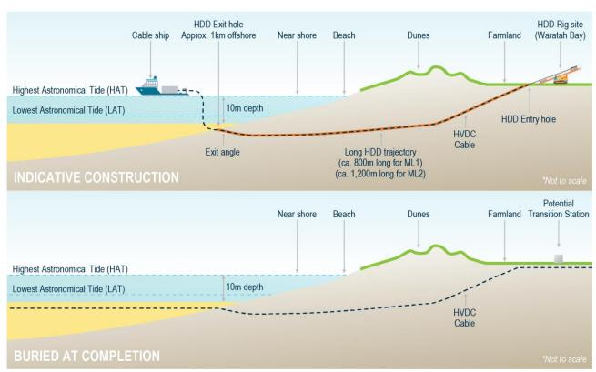
Figure 4.3: Long trajectory HDD proposed for Victorian shore crossing
