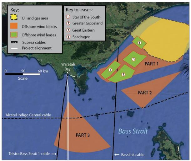
Source: Google Earth™, Tetra Tech Coffey Webmap, DCCEEW (2023c). Note map is for illustrative purposes. Widths of the telecommunication cables and HVDC cables are enlarged for visibility. The oil and gas area denotes the 'Area to be Avoided' (DCCEEW, 2022h).
