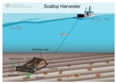
Figure 14. Scallop dredge method diagram (image source: afma.gov.au).
