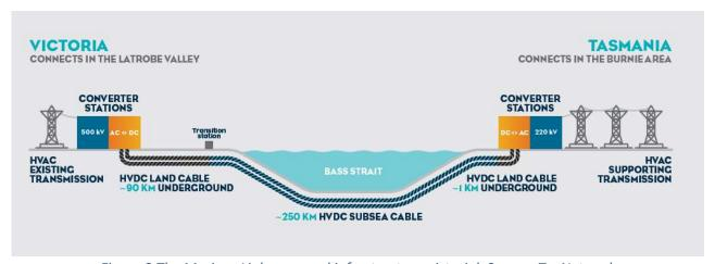
Figure 3 The Marinus Link proposed infrastructure pictorial, Source: TasNetworks
