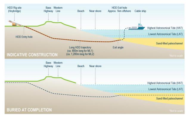
Figure 4.2: Long trajectory HDD proposed for the Tasmanian shore crossing
