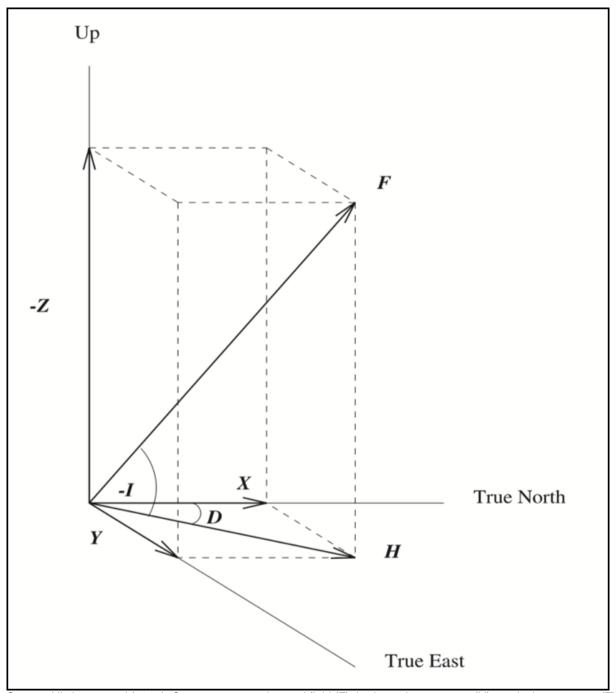
Source: Hitchman et al (2000). Components are the total field (F), horizontal component (H), vertical component (Z), north component (X), east component (Y), declination(D), and inclination (I). The orientation of the vertical component, which results in both Z and I having negative values, describes the magnetic field direction in the Southern Hemisphere.
