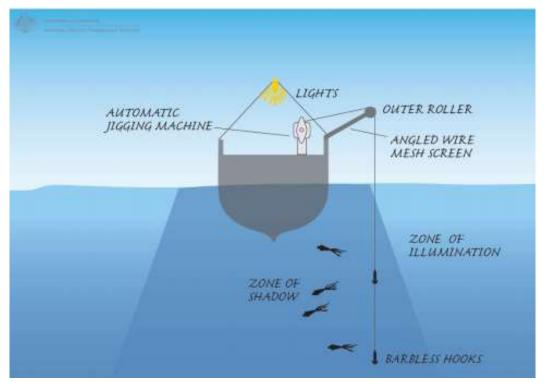
Figure 11. Squid jig method diagram (image source: afma.gov.au).
