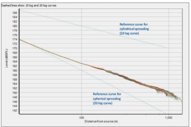
Source: MDA (2022). The two blue dashed curves depict the reduction for spherical and cylindrical sound propagation.
