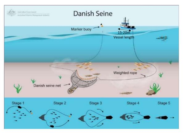
Figure 6. Danish seine method diagram (image source: afma.gov.au, with edits)
