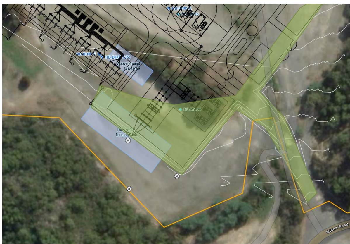
Figure 4-2: Proposed new groundwater monitoring locations and approximate extent of bulk earthworks cut (green) (PFAS source areas – Synnot & Wilkinson, 1996)
